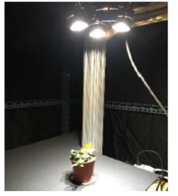
Figure 3. Obtaining images with hyperspectral imaging system
